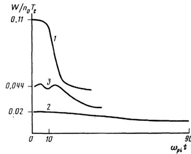
FIG. 2. Time-dependence of the average energy density of the field in the caviton: 1  $\epsilon/\epsilon_0 = 6.6$ ; 2: 1.25; 3: 2.7.
