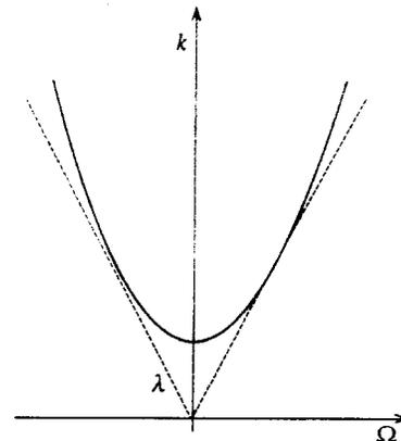
FIG. 2. Dispersion curve (3.23) for positive  $\lambda$ . The dashed lines which are tangent to the dispersion curve correspond to the critical velocities  $\beta = \pm 2\sqrt{\lambda}$ . These straight lines specify the boundary of the soliton cone of angles.
