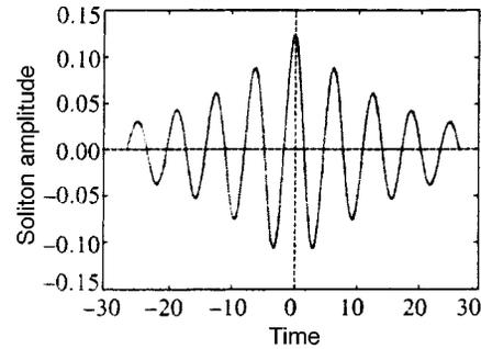
FIG. 4. Dependence of the soliton amplitude (in units of  $\nu_0^2$ ) on the time (in units of  $\nu_0^{-1}$ ) for  $\mu/\nu_0 = 1/3$ . The soliton envelope has the form of the function  $\text{sech}$  to good accuracy.
