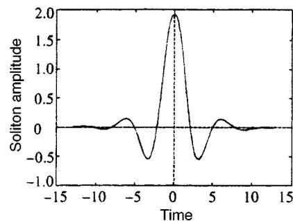
FIG. 5. Form of a soliton when  $\mu/\nu_0 = 1$ . The amplitude of the soliton (in units of  $\nu_0^2$ ) increases, and its width (in units of  $\nu_0^{-1}$ ) decreases. Oscillations are still observed on the scale of the soliton.
