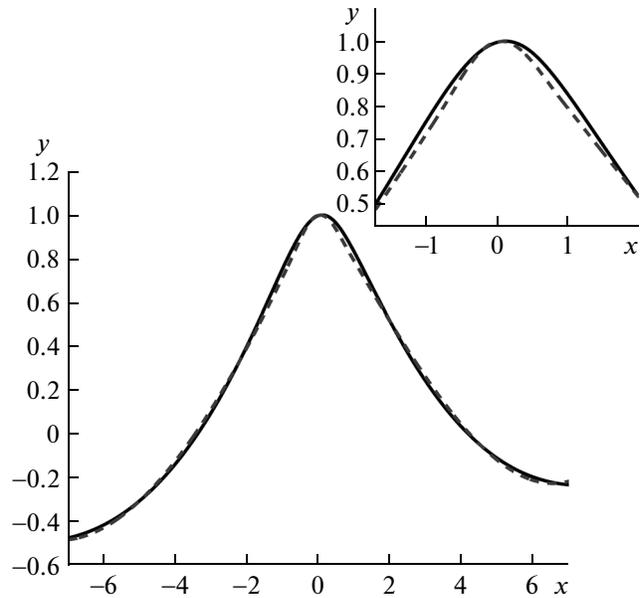
**Fig. 2.** Approximation of the profile with cubic polynomials.
